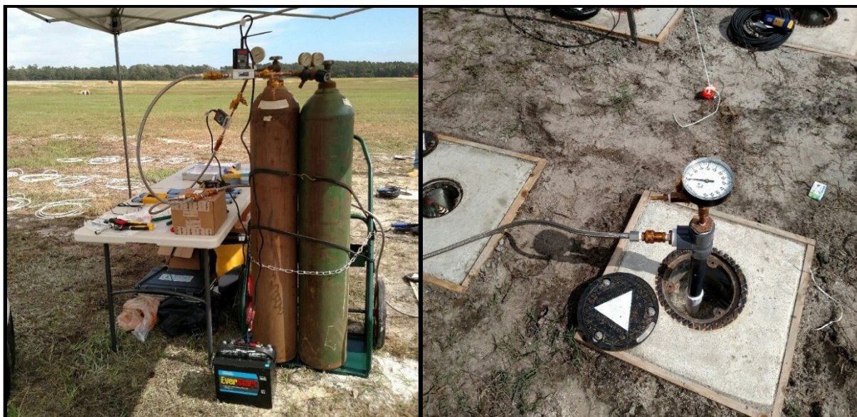
Figure 5.7. Photographs of Sparge Testing Setup
