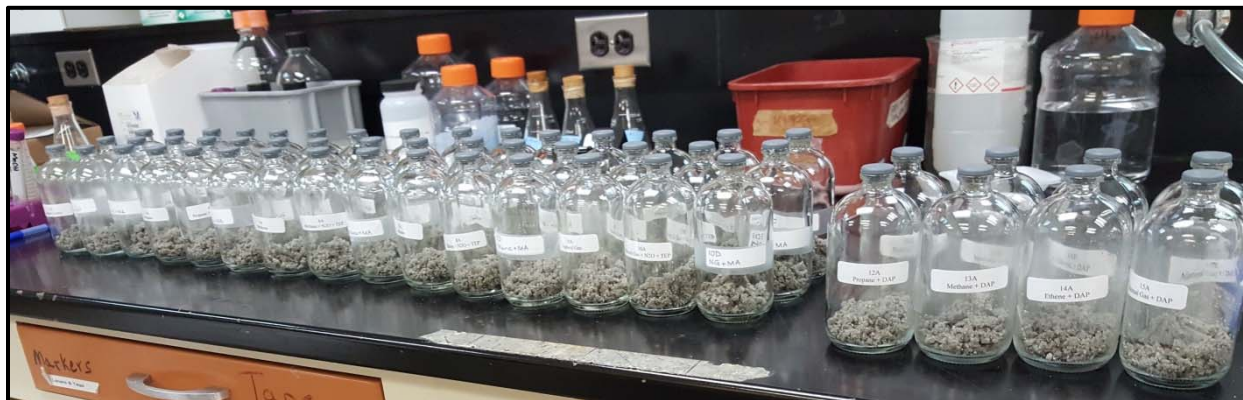
Figure 3.1. Photograph of Homogenized Soil Added to Serum Bottles
