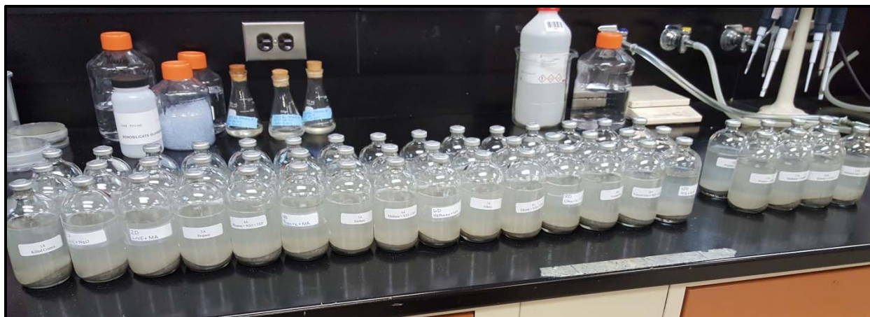
Figure 3.2. Photograph of Microcosms Set Up With Site Soil and Groundwater
